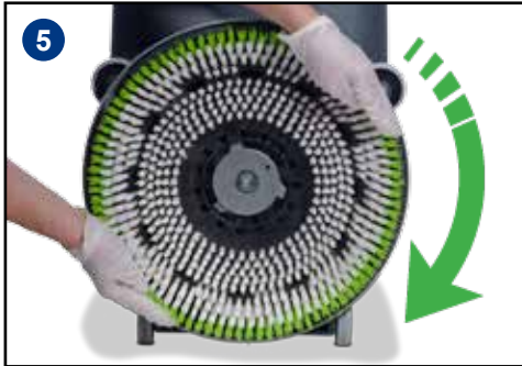
Fit the brush / pad to the drive chuck, twist to lock the brush (Fig.5) / pad in place (Fig.6).
