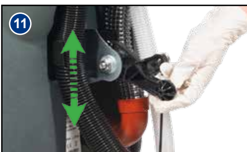
Raise the floor-tool for transit or lower for cleaning operation using the lifting handle fitted to the back of the machine (Fig.11).
