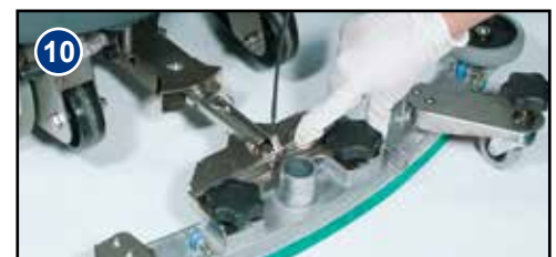
Fit the floor-tool and retain using the detent pin (Fig.9).
