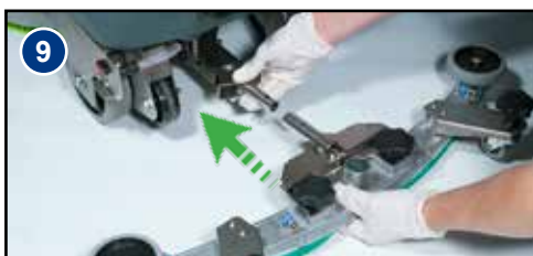
Fit the floor-tool and retain using the detent pin (Fig.9).
