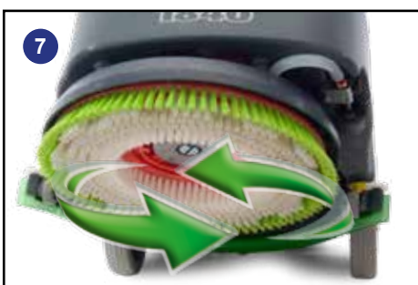
Fit the brush / pad onto the Nulock drive chuck, twist to lock the brush / pad in place (Fig 7).
